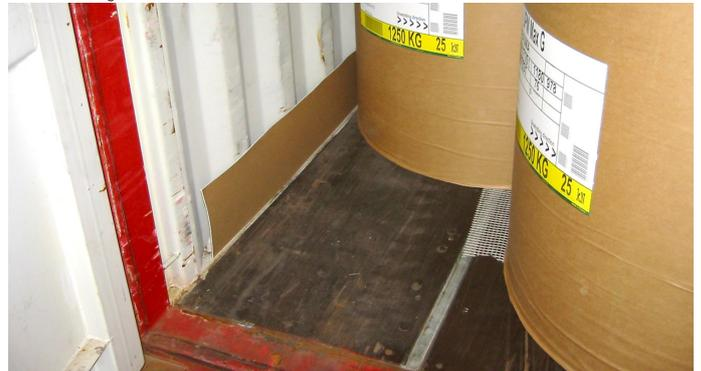
Uneven walls and floors in containers and trains may cause transport damage to the loaded goods. This can be avoided by using Flatboards as side and floor protection.
