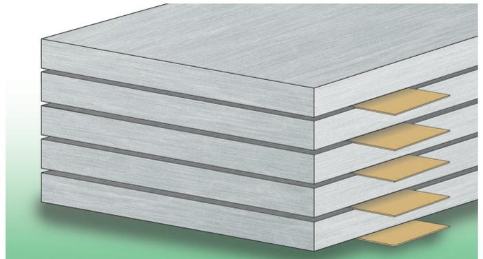
Using flatboards in between very delicate laminate products prevents all scratches.
